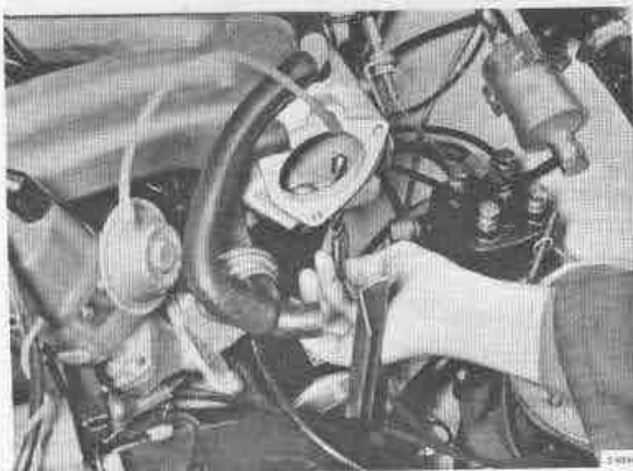
CLEANING THE HOLE IN THE INLET MANIFOLD WALL
