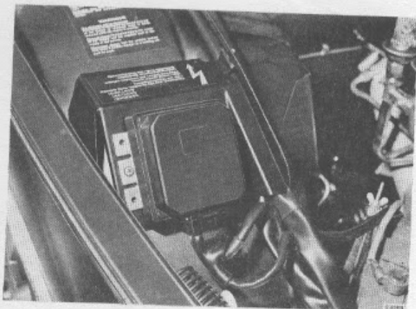
ELECTRONIC CONTROL UNIT
