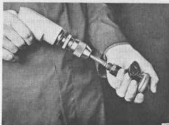
CLEANING THE INLET OF THE EGR VALVE
