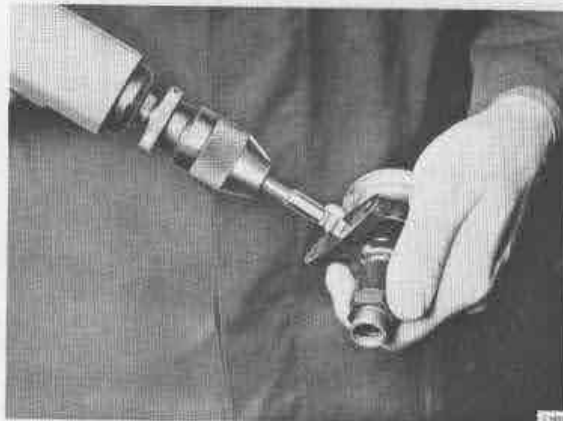
CLEANING THE OUTLET OF THE EGR VALVE
