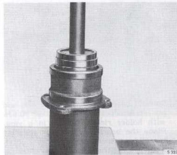
Pinion shaft with bearing, bearing housing and spacer sleeve.
