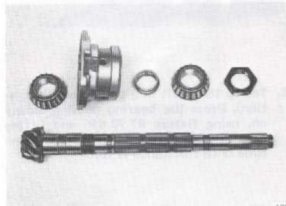
Pinion shaft with bearing, bearing housing and spacer sleeve.
