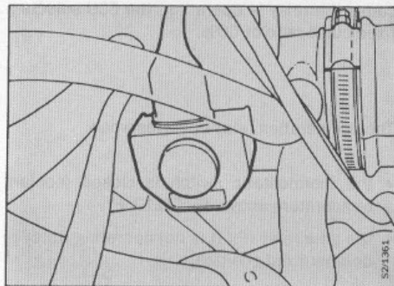
Throttle-position sensor on normally aspirated engine
