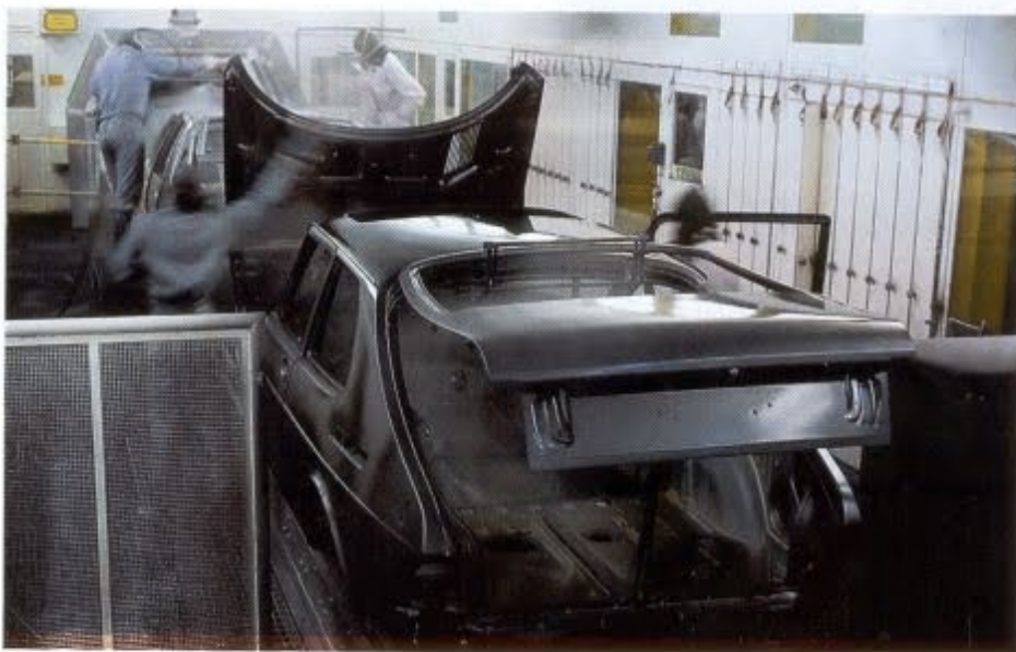
Two coats are applied for metallic finishes. The first coat is thin and has a high pigment content. The last coat is a thick layer of clear varnish which protects the pigment and produces a very high gloss.
