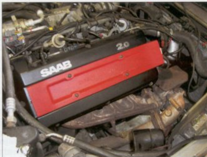
Saab DI Cassette installed on a Classic 900.
