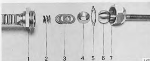
BALL JOINT, DISASSEMBLED
