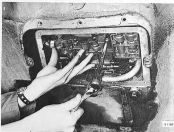
SCREWING ON THE VALVE HOUSING
