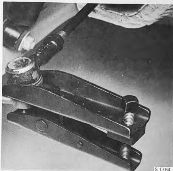
REMOVING THE STEERING ARM Tool 899540
