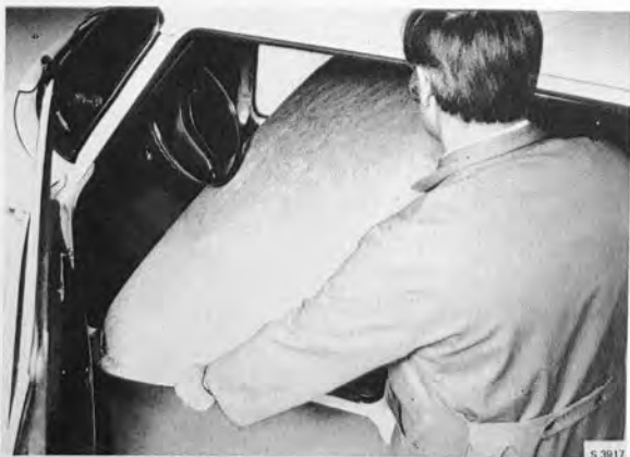
THE LINING IS LIFTED OUT THROUGH LEFT DOOR
