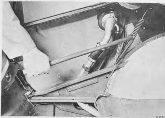
REMOVAL OF SPRING, TRUNK LID Tool 829157
