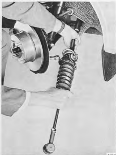
REMOVAL OF STEERING GEAR ASSEMBLY
