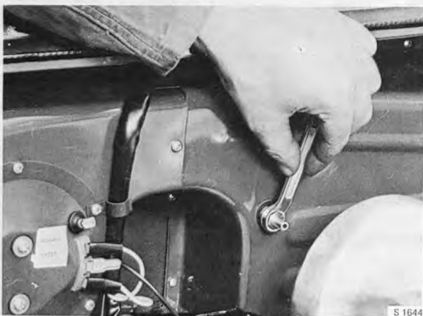
THE HEAT EXCHANGER BLEEDER NIPPLE, UP TO AND INCL. MODEL 1973
