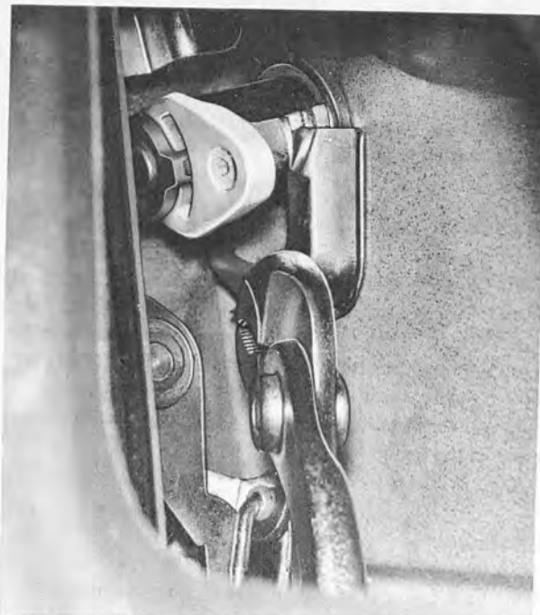
THE LOCK CLIP IS REMOVED
