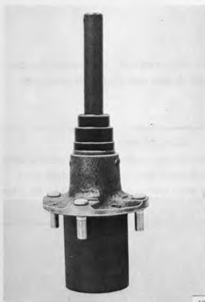
PRESSING IN THE SEAL RING Tool 899516
