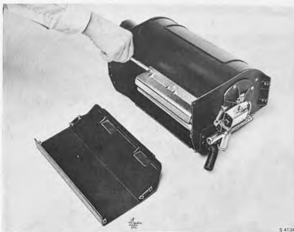
THE HEAT EXCHANGER RETAINING PLATE IS REMOVED
