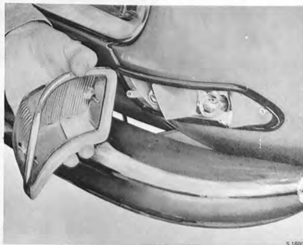
CHANGING BULBS, FRONT, UP TO AND INCL. MODEL 1971
