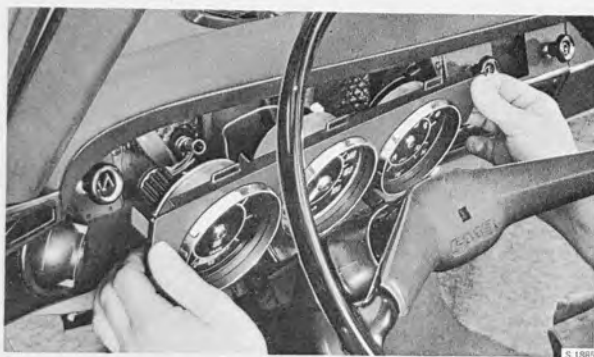
REMOVING THE INSTRUMENT UNIT
