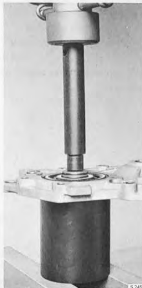
PRESSING OUT THE OUTPUT GEAR FROM THE BEARING Drift 839018, support 839009
