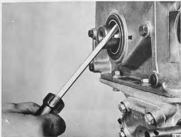
REMOVING THE SEAL RING AT THE TRANSMISSION END
