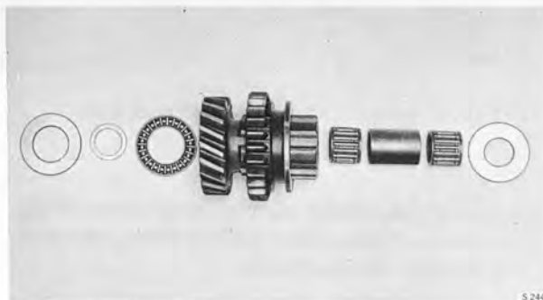
REVERSE GEAR WITH BEARINGS AND WASHERS
