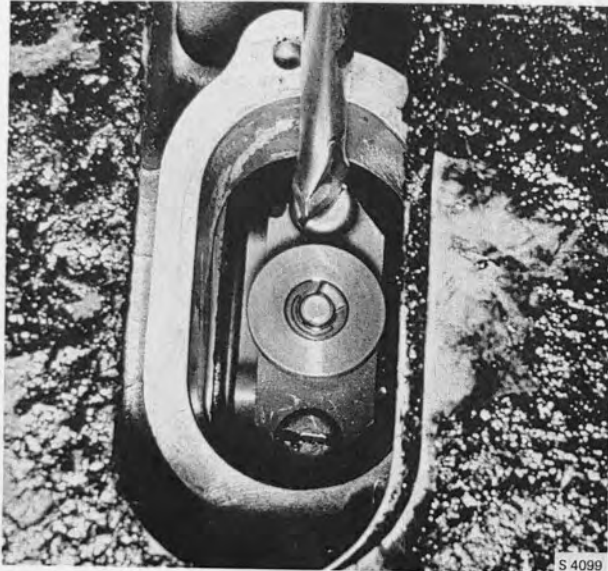
THE GOVERNOR SCREWS ARE REMOVED
