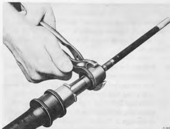
REMOVING OUTER BEARING CUP AND LOCK NUT Tool 839019 and polygrip pliers
