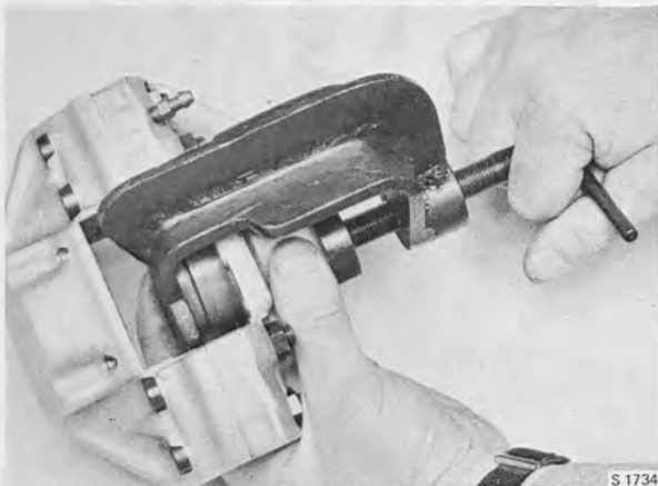
PUSHING THE BRAKE PISTON INTO THE CYLINDER Tool 786043
