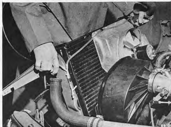
REMOVING THE FRONT SHEET
