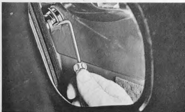
TAKING OFF THE SNAP RING
