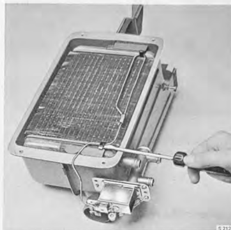
FREEING THE THERMOSTAT COIL
