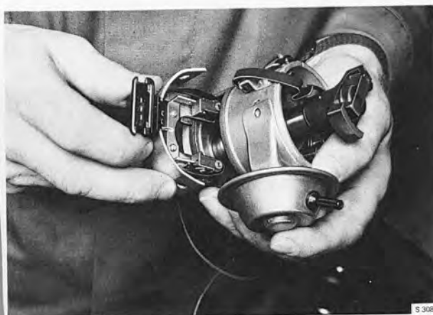
REMOVING THE IMPULSE CONTACTS
