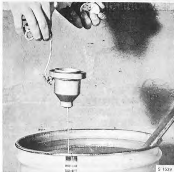
MEASURING VISCOSITY WITH AN SIS BEAKER
