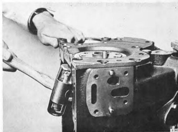
REMOVING THE GABLE PLATE
