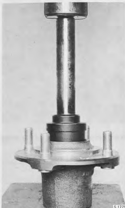
PRESSING IN THE BEARING OUTER RINGS Tool 899516
