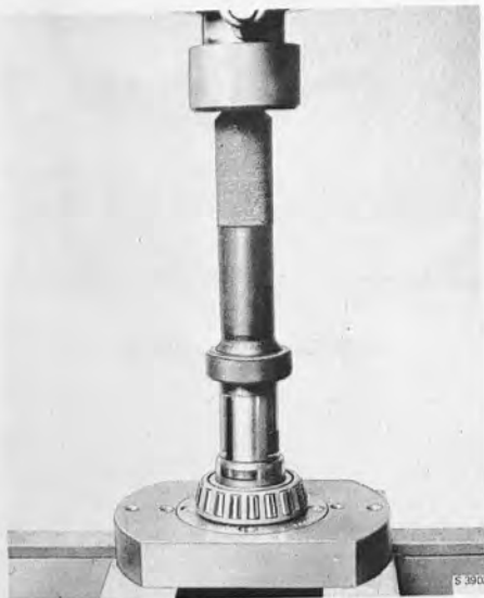
PRESSING OFF THE REAR PINION BEARING Tools 879063 and 879065 alt. 879066
