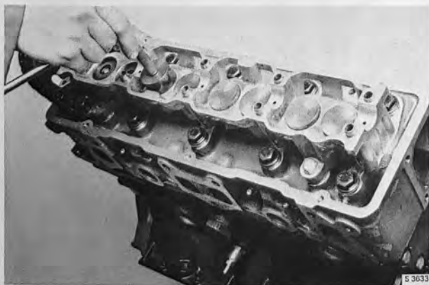
REMOVING THE VALVE DEPRESSORS Tool 839140
