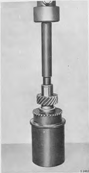
PRESSING ON THE FREE WHEEL DRIVER GEAR Drift 839018, supports 839009 and 839024
