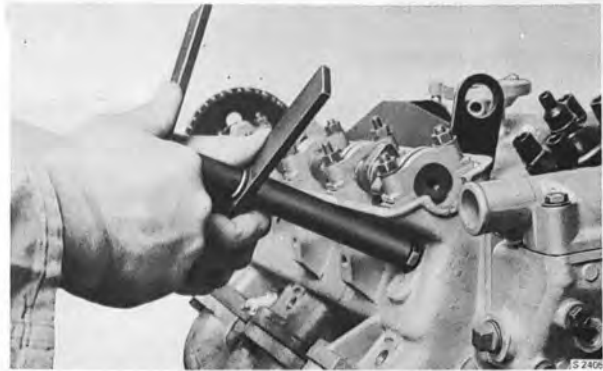
REMOVING STUDS Tools 839051 and 839052
