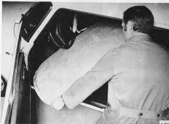
THE LINING IS LIFTED INTO THE CAR
