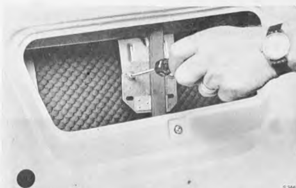
REMOVING SCREWS FROM THE WINDOW RETAINER
