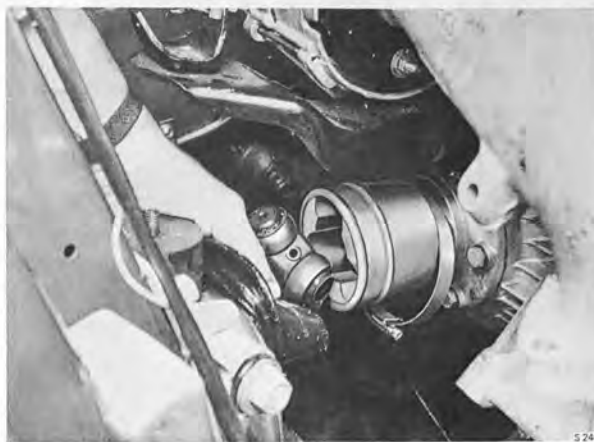
ASSEMBLING THE RIGHT INNER UNIVERSAL JOINT
