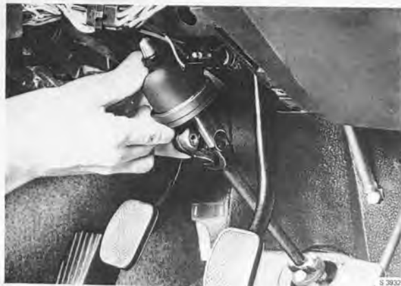
INSTALLATION OF SEALING BELLOWS, INTERMEDIATE SHAFT
