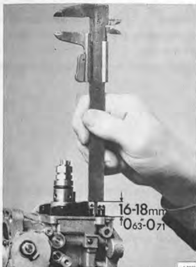
MEASURING FLOAT LEVEL
