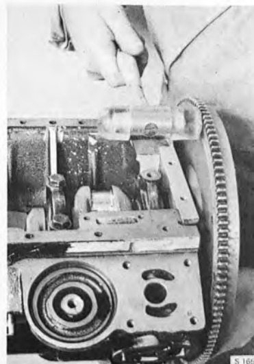
REMOVING THE FLYWHEEL
