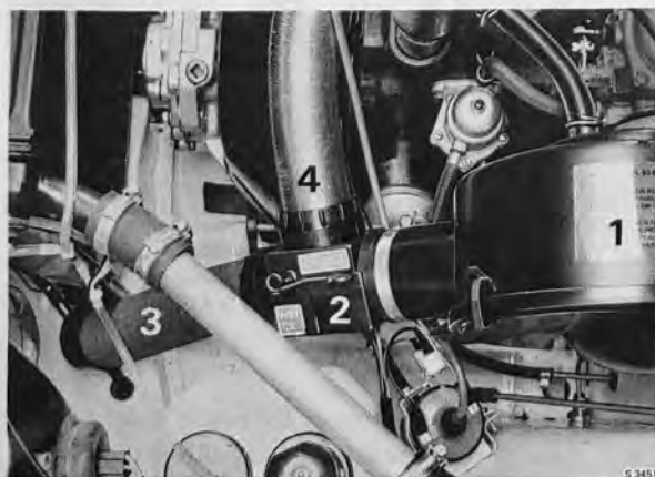
AIR CLEANER WITH HOSES, CARBURETED ENGINE MODEL 1972
