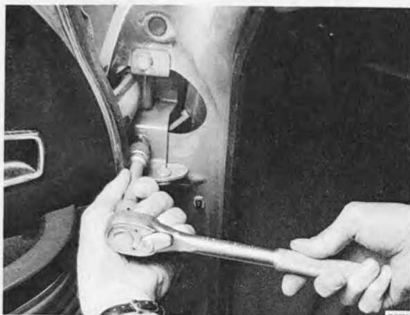
UNSCREWING THE DOOR HINGES
