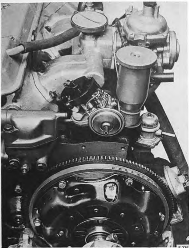
POSITION FOR INSTALLING THE ROTOR, DISTRIBUTOR FULLY ENGAGED
