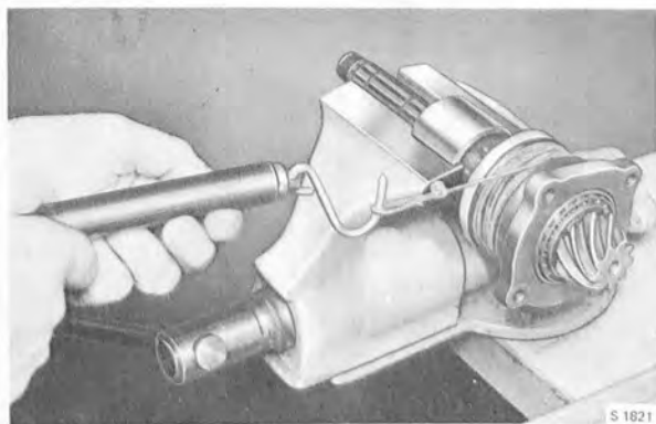
CHECKING THE BEARING HOUSING TORQUE Tools 839006 and 839013
