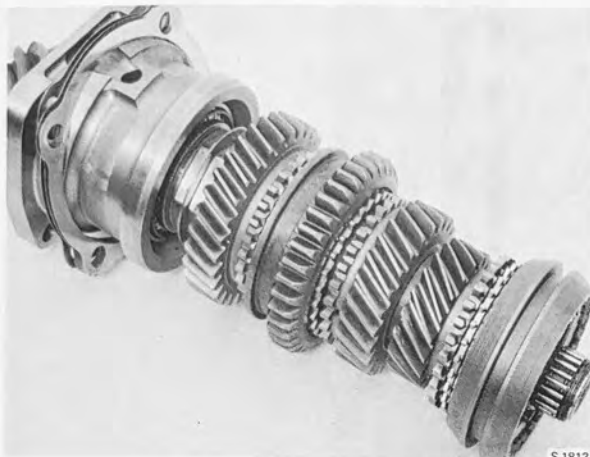
PINION SHAFT WITHDRAWN
