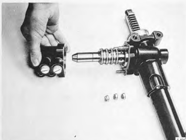
FITTING THE VALVE HOUSING. THE VALVE SHAFT IS FITTED WITH FITTING CONE
