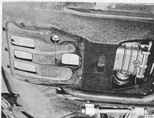
DRAIN PLUGS, AUTOMATIC TRANSMISSION
