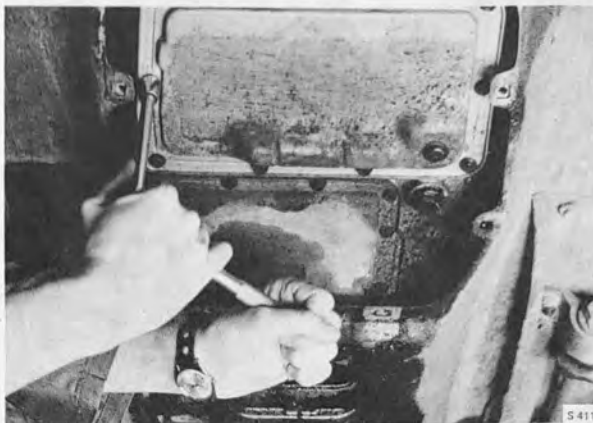
THE BOTTOM COVER IS INSTALLED
