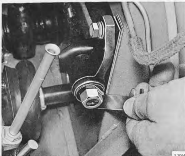
LOCATION OF CAMBER ADJUSTMENT SPACERS
