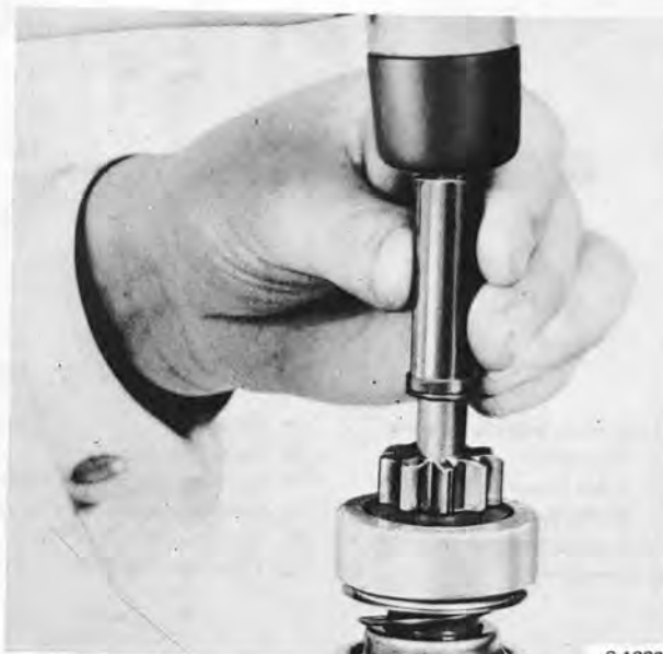
PUSHING DOWN THE STOP RING
