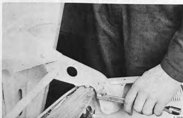
UNDOING HOOD FASTENING SCREWS
