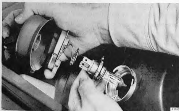
CHANGING A HEADLIGHT BULB, HALOGEN TYPE
