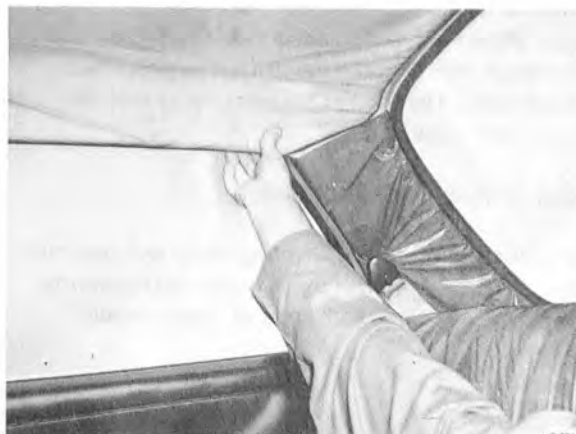
THE REAR EDGE IS POSITIONED
