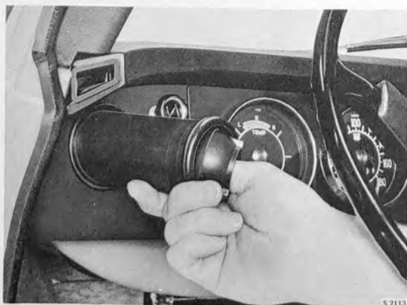
REMOVING THE FRESH AIR BLOWER NOZZLES
