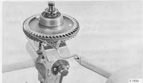
COMPRESSING THE CENTER SHAFT BEARINGS Dynamometer 839013
