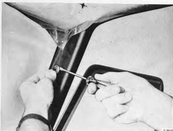
THE SAFETY PADS ARE REMOVED FROM THE WINDOW PILLARS
