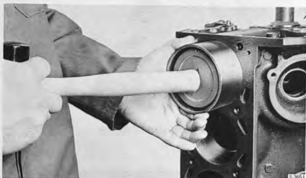
INSTALLING PISTON AND CONNECTING ROD Tool 786228
