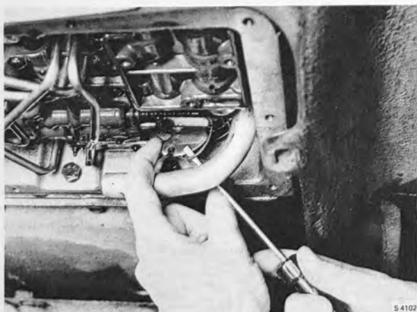
DISCONNECTING THE THROTTLE WIRE
