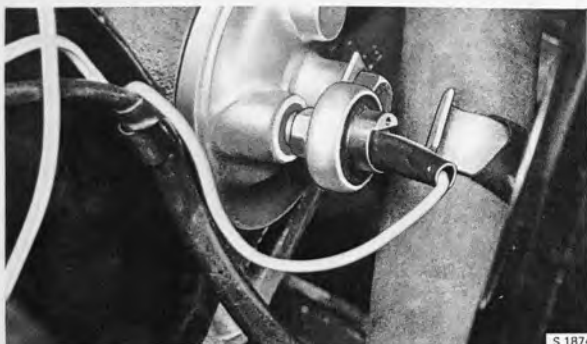
OIL PRESSURE SWITCH, 1.7 AND 1.85 L ENGINES
