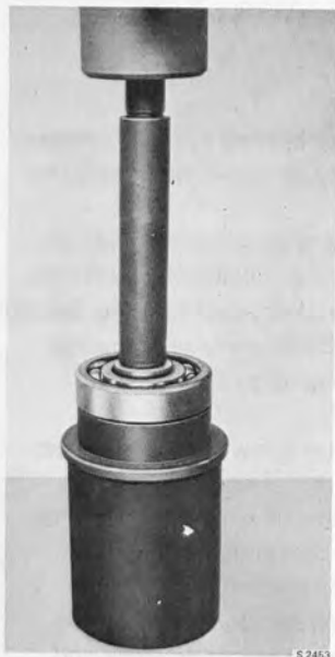
PRESSING THE INPUT GEAR OUT OF THE BEARING
