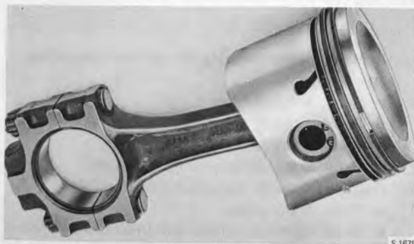
PISTON AND CONNECTING ROD
