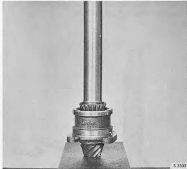
PRESSING IN THE FRONT ROLLER BEARING Tool 839014
