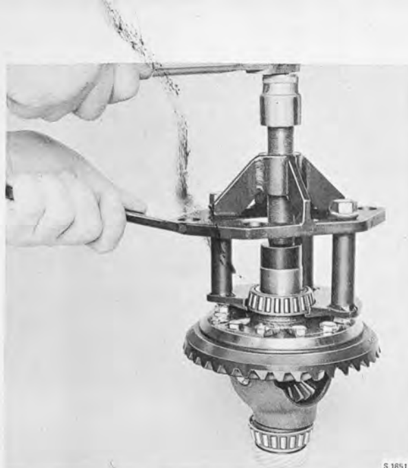
REMOVING DIFFERENTIAL JOURNAL BEARINGS Puller 899518, 899525, wheel nuts 890914
