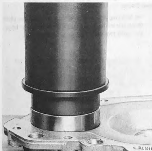
PRESSING IN THE GEAR AND BALL BEARING IN THE BEARING HOUSING
