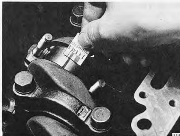
READING THE CLEARANCE
