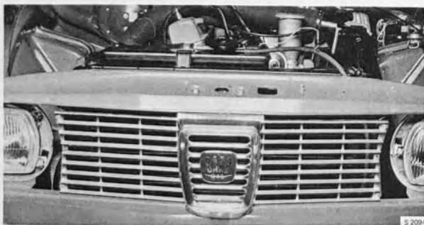
GRILLE WITH HEADLIGHT TRIM FRAMES REMOVED
