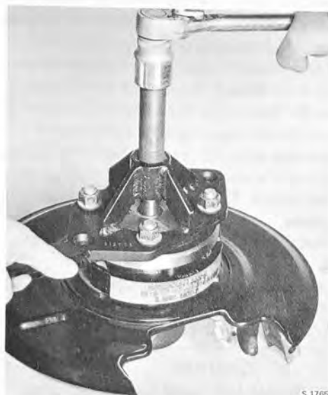
REMOVING THE WHEEL HUB Tool 899518
