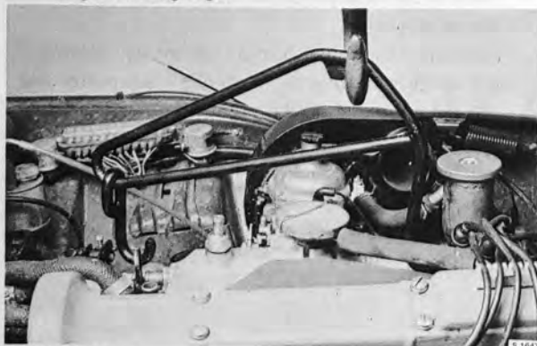
LIFTING YOKE Tool No. 839097
