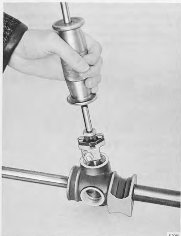
REMOVING THE PINION Tools 839027 and 899528
