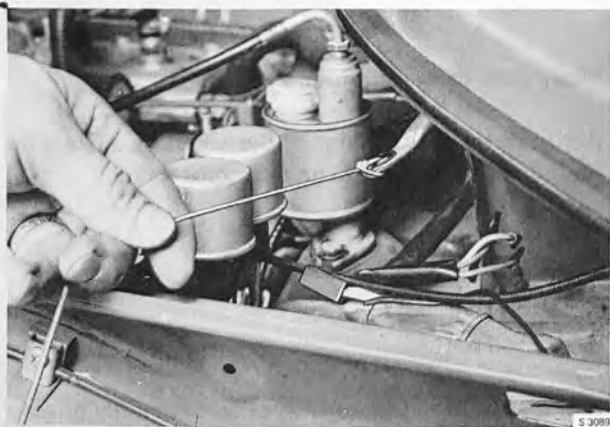
TYING A STRING TO THE WIPER LINKAGE
