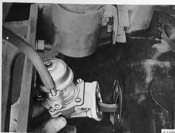
INSTALLING THE FUEL PUMP
