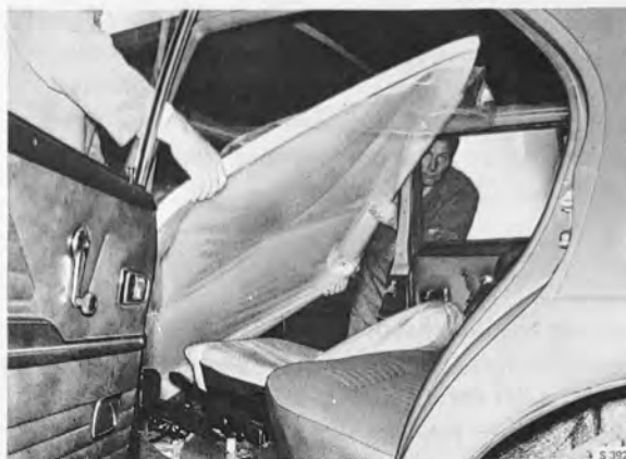
THE LINING IS MOVED IN, 4-DOOR MODEL
