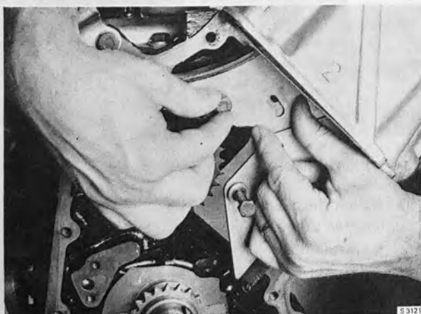
MOUNTING THE CURVED CHAIN GUIDE PLATE
