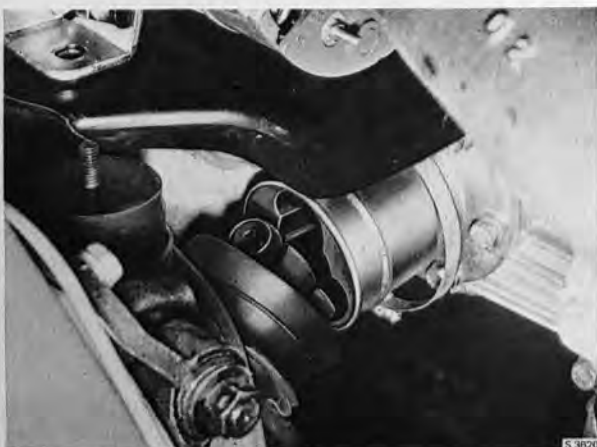
ASSEMBLING THE RIGHT INNER UNIVERSAL JOINT
