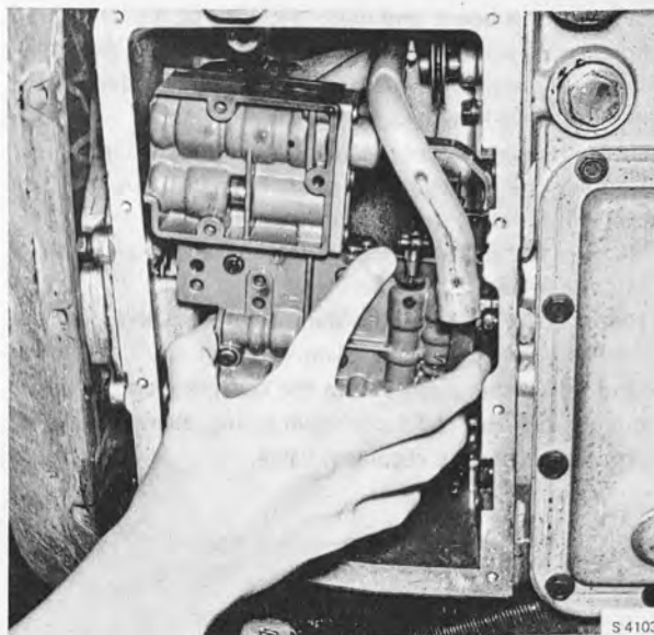
LIFTING OUT THE VALVE HOUSING
