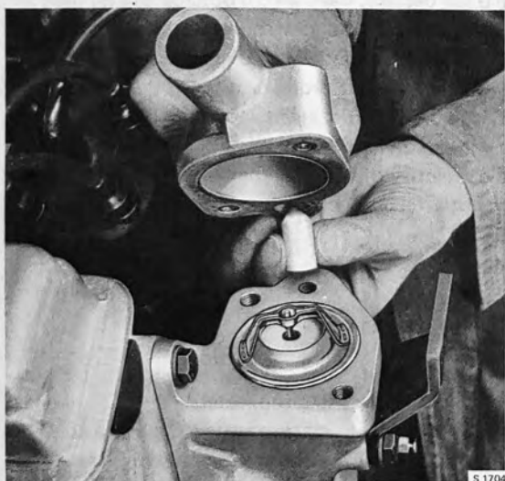
THERMOSTAT HOUSING WITH THERMOSTAT, WATER OUTLET PIPE AND VALVE BODY (Valve body only up to and incl. model 1970.)
