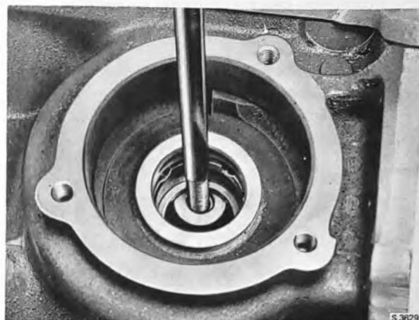
REMOVING THE BEARING HOUSING Tool 839027
