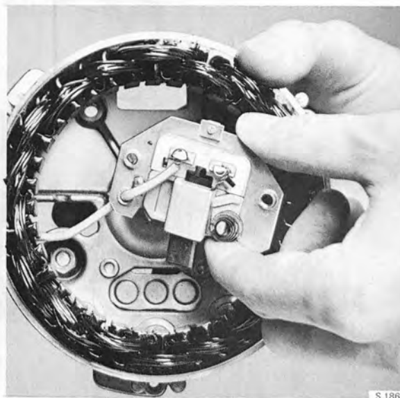
REMOVING THE BRUSH UNIT ASSEMBLY
