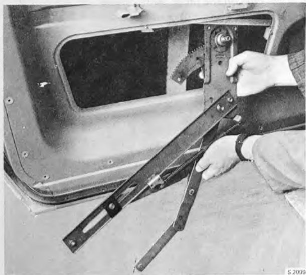
REMOVING THE WINDOW REGULATOR
