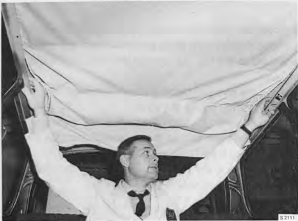
INSTALLING THE CROSS RIBS
