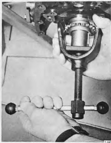
DISASSEMBLING THE CRANKSHAFT SPROCKET PULLER No. 839185
