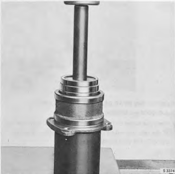
INSTALLING THE BEARING RACE IN BEARING HOUSING Tools 839018 and 879046
