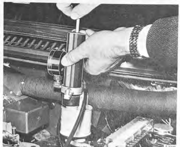
BLEEDING THE CLUTCH SYSTEM
