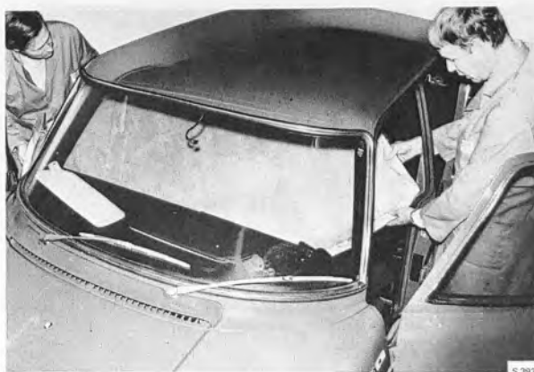
THE LINING IS MOVED INTO POSITION IN THE CAR
