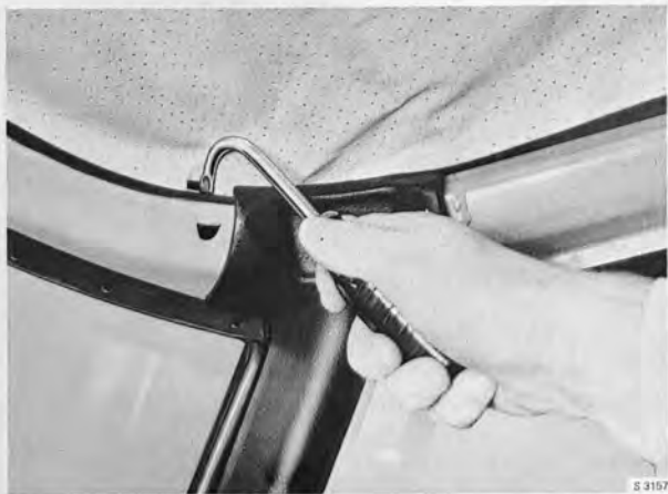
HOOKING THE HEADLINING TO THE FORWARD CORNERS Tool 829058
