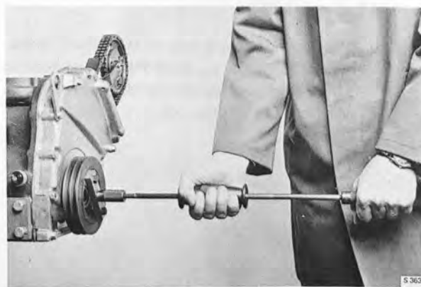
REMOVING THE BELT PULLEY Tools 839027 and 839215
