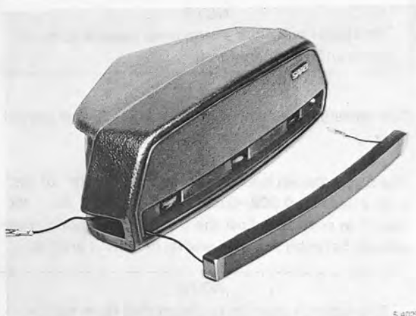
HORN CONTACT DISCONNECTED FROM SAFETY PAD (MODEL 1974)
