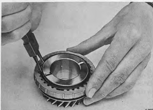
REMOVING THE SYNCHRONIZING RING FOR 3RD GEAR
