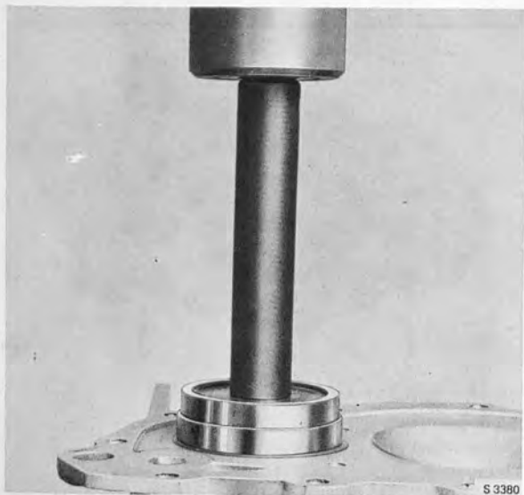
PRESSING OUT THE BEARING FROM THE BEARING HOUSING Tools 839018 and 839046
