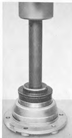
SEATING THE OUTER BEARING RINGS
