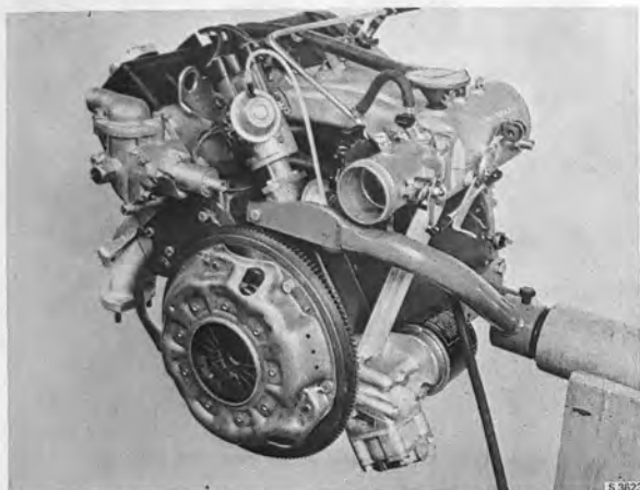
ENGINE MOUNTED IN WORK STAND Tool 839216
