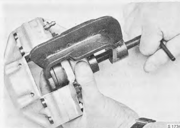
PUSHING THE BRAKE PISTON INTO THE CYLINDER
