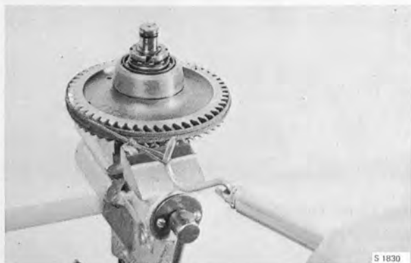
COMPRESSING THE CENTER SHAFT BEARINGS Tool 839013
