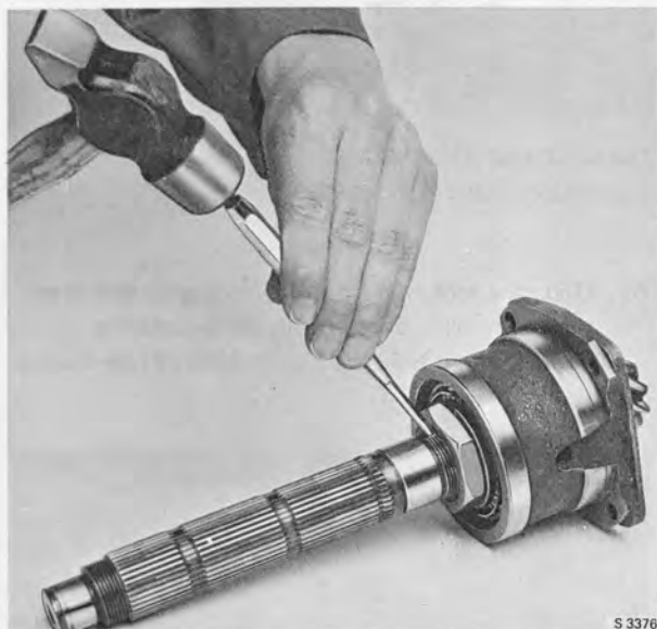
LOCKING THE PINION BEARING NUT
