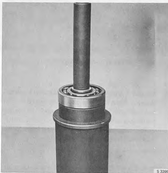
PRESSING THE BEARING OFF THE INPUT GEAR Tools 839018, 839009 and 839024
