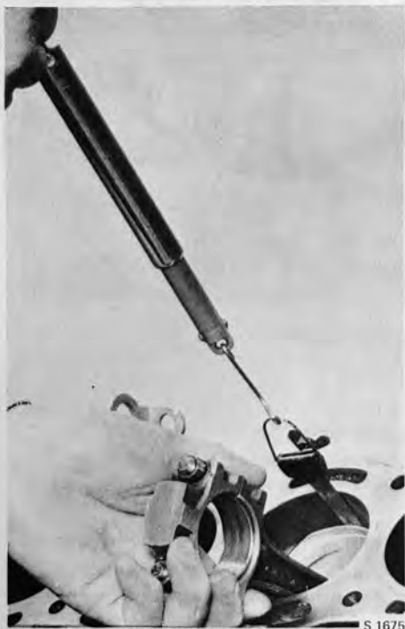
MEASURING PISTON CLEARANCE
