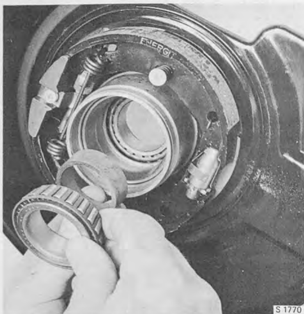
FITTING THE INNER RINGS OF THE BEARINGS
