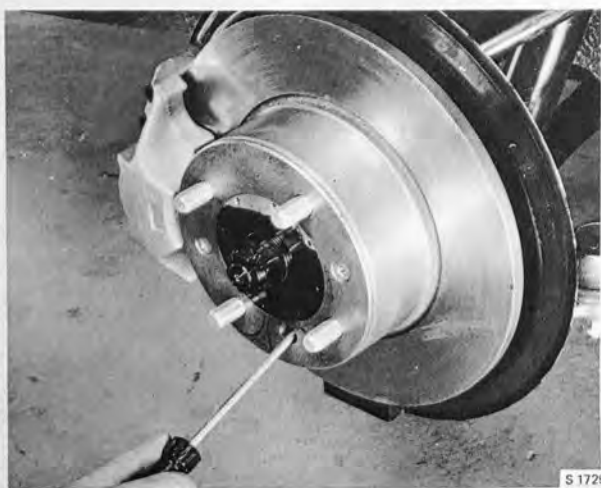
RELEASING THE BRAKE SHOES
