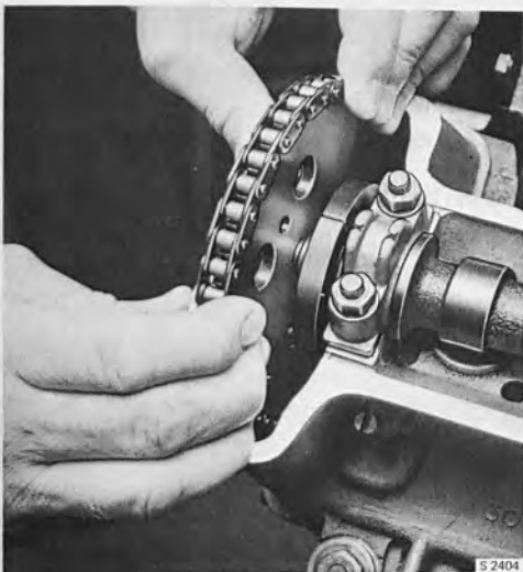
SEPARATING THE CAMSHAFT CHAINWHEEL FROM THE CAMSHAFT PLATE
