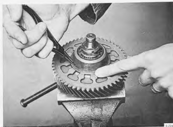
MOUNTING THE FRICTION WHEEL
