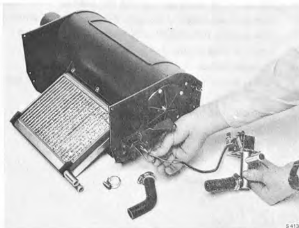
THE THERMOSTAT IS REMOVED
