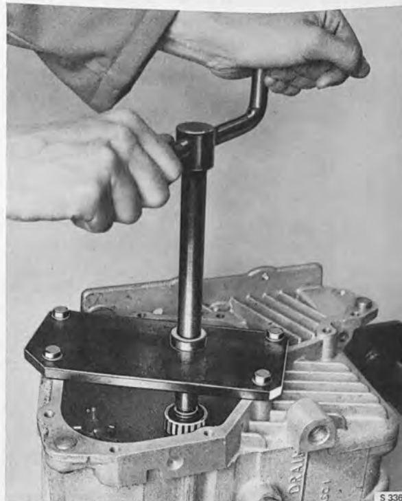
PRESSING OUT THE PINION SHAFT Tool 879051
