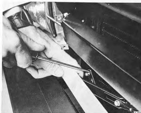
LOOSE THE CRANK ARM FROM THE PUSH ROD
