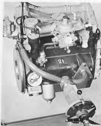
ENGINE MOUNTED IN WORK STAND Tool 839045
