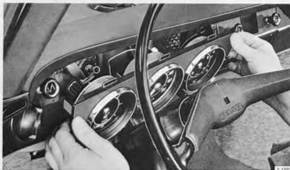
REMOVING THE INSTRUMENT UNIT
