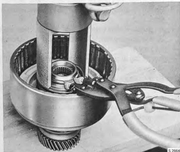
REMOVING LOCK RING IN REAR CLUTCH, Tools 879008 and 879018
