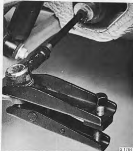
REMOVING THE STEERING ARM Tool No. 899540
