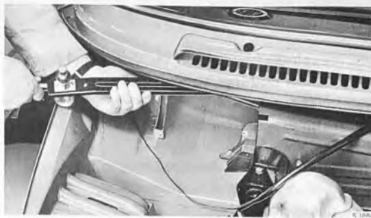
REMOVING THE WIPER MECHANISM
