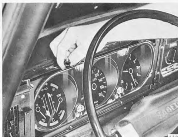
CHANGING INSTRUMENT ILLUMINATION LIGHT BULB
