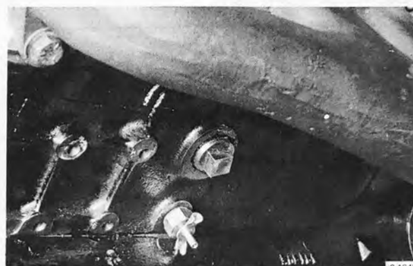
ENGINE BLOCK DRAIN COCK
