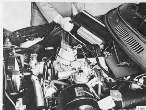
REMOVING THE FAN CASING
