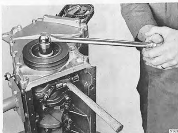
REMOVING THE BELT PULLEY SCREW
