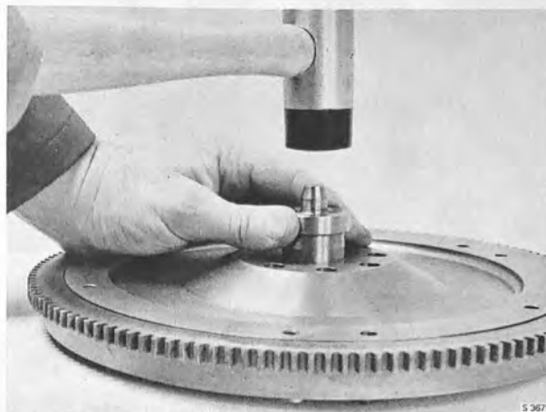
REMOVING THE CLUTCH SHAFT BEARING Tool 839199
