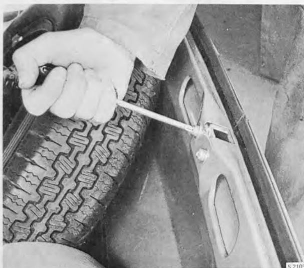
ADJUSTING THE STRIKER PLATE
