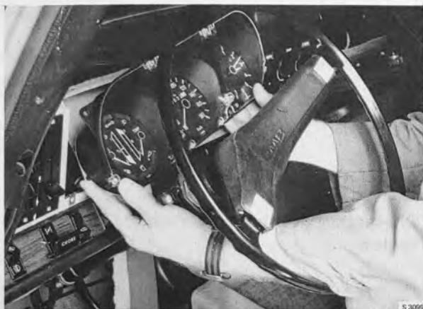
REMOVING THE INSTRUMENT UNIT, 1971 MODEL
