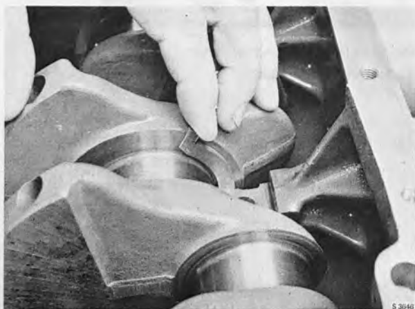
INSTALLING THE THRUST BEARING
