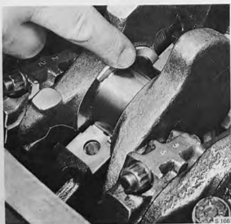
POSITION OF THRUST BEARING WASHERS
