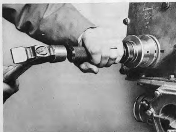
FITTING THE SEAL RING, TRANSMISSION END Tools 839044 and 839188
