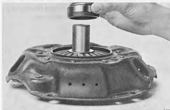
CENTERING OF RELEASE BEARING
