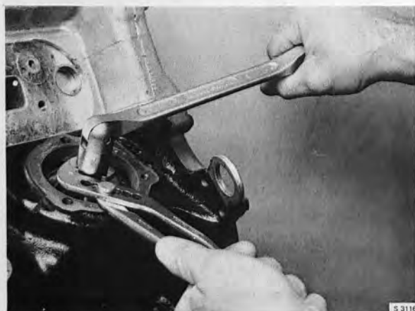
UNDOING THE CENTER SCREW OF THE WATER PUMP
