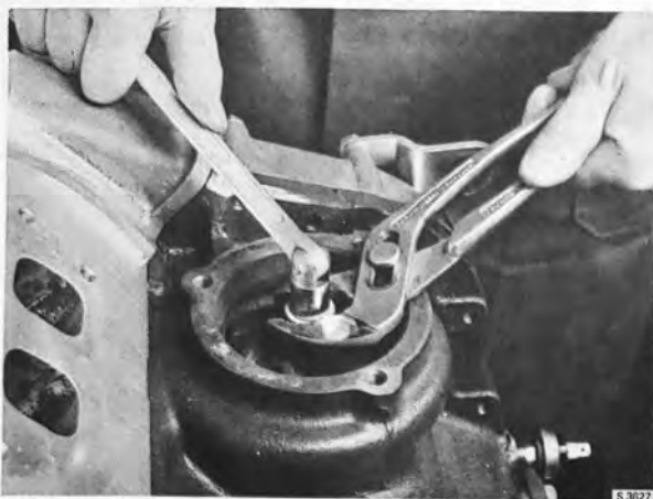
UNDOING THE CENTER SCREW OF THE WATER PUMP
