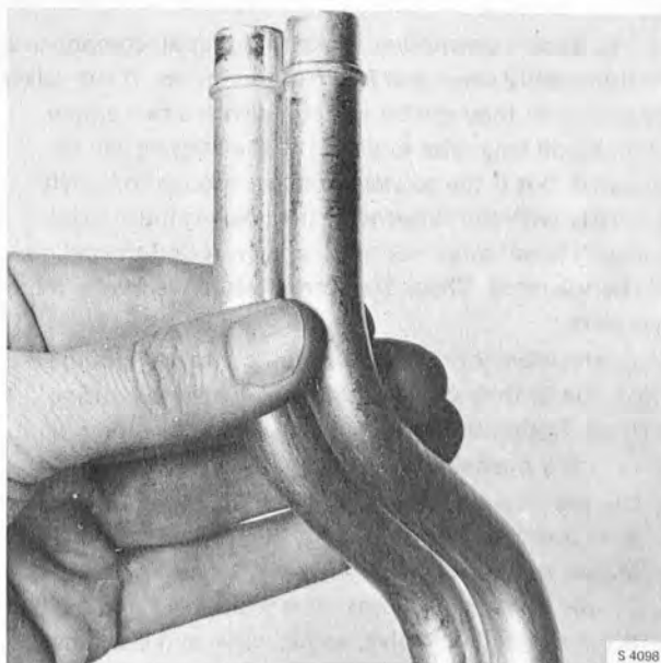
CHECKING THE OIL PIPE
