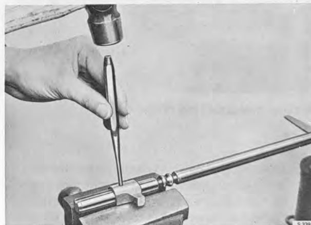
REMOVING THE COTTER PIN FROM THE DRIVER
