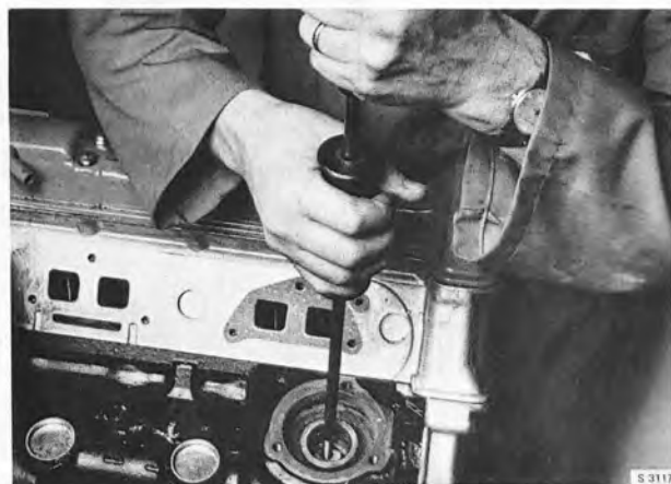
REMOVING THE BEARING HOUSING Tool 839027
