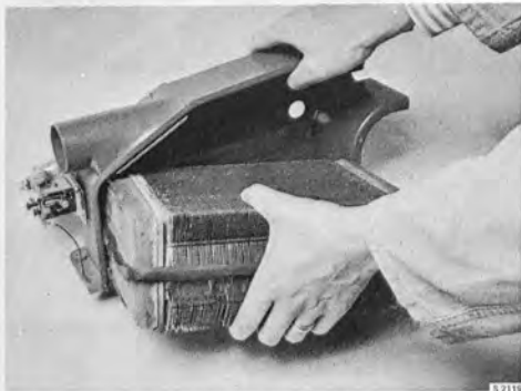
SEPARATING THE HEAT EXCHANGER CASING
