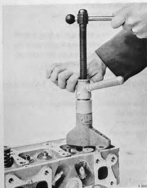
REMOVING THE VALVE GUIDE Tool 839043
