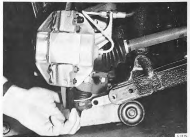
UNDOING LOWER END PIECE FROM CONTROL ARM
