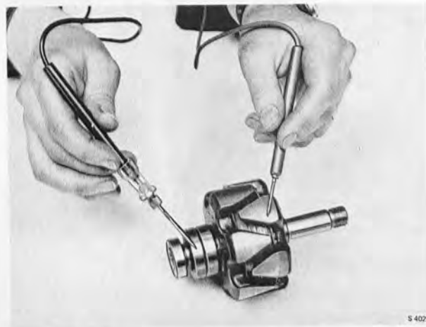
CHECKING THE INSULATION OF THE EXCITER WINDING AND THE SLIP RINGS
