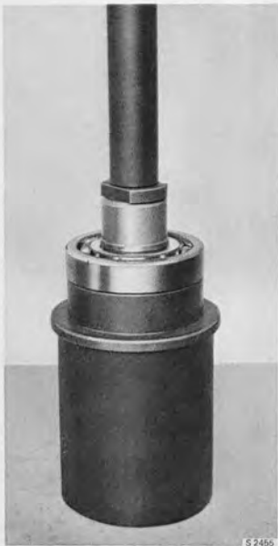
PRESSING OFF THE BEARING
