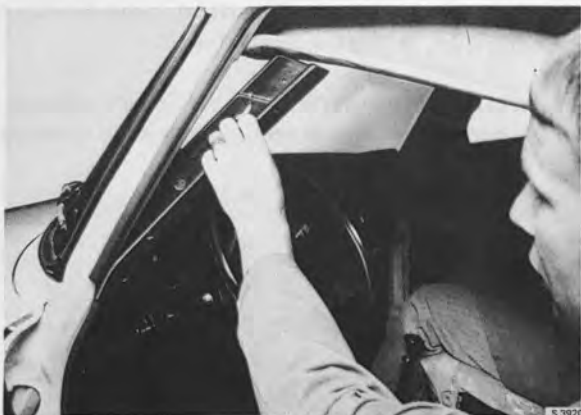
THE FRONT DOOR PILLAR PADS ARE INSTALLED
