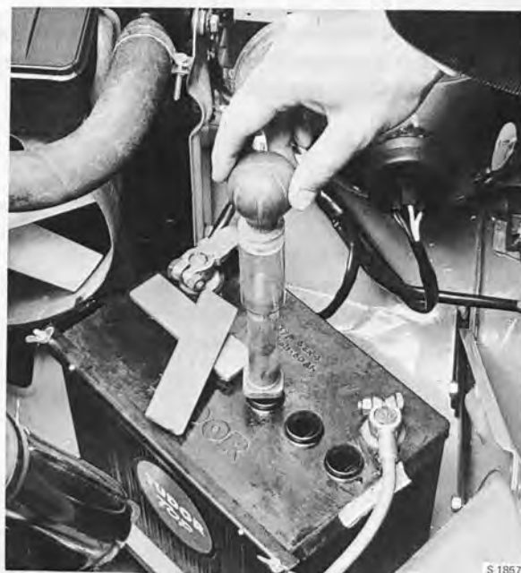
TESTING THE BATTERY
