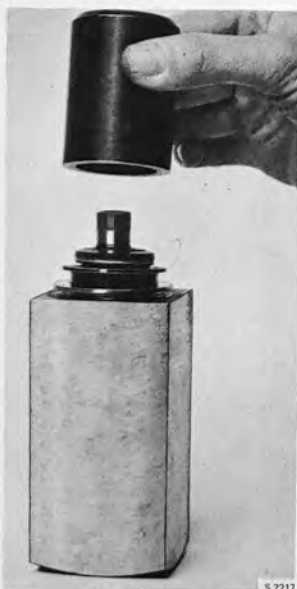
FITTING THE WATER PUMP SEAL Tools 839053 and 839054
