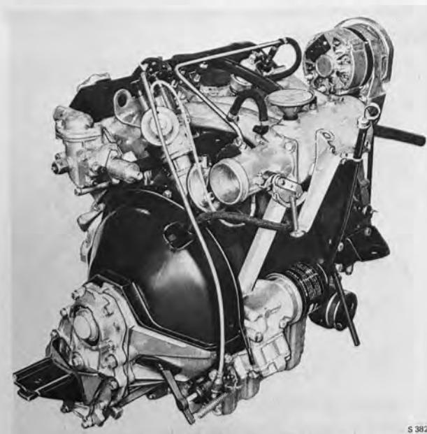
POWER PLANT, 2.0 L INJECTION ENGINE WITH MANUAL TRANSMISSION
