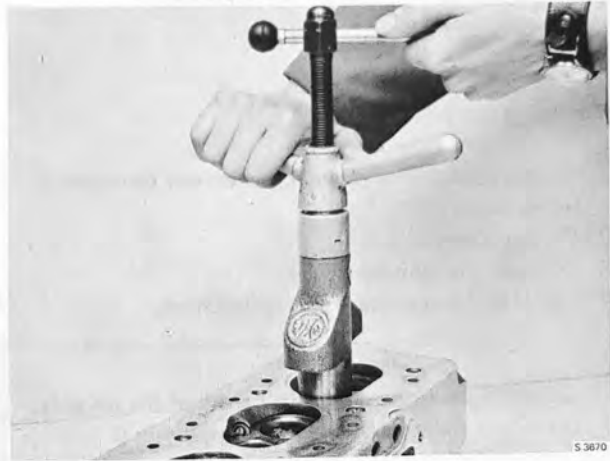
INSTALLING THE VALVE GUIDE Tool 839043
