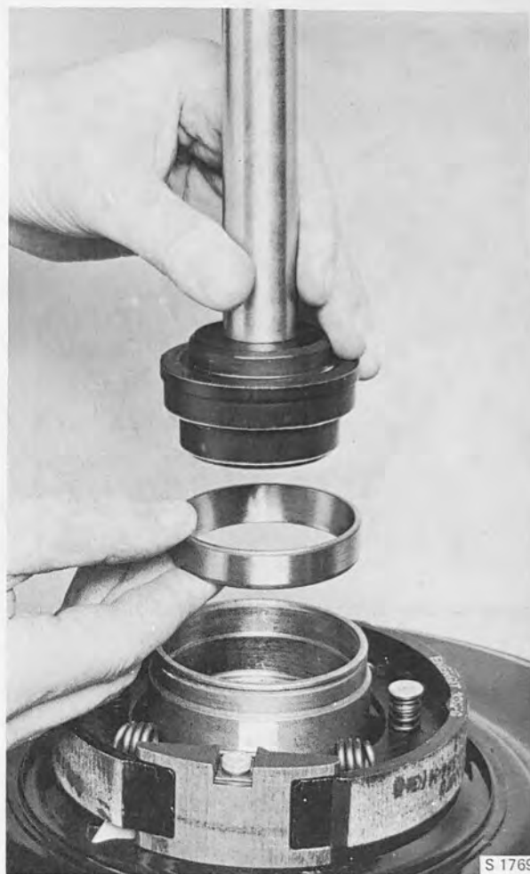
PRESSING IN THE OUTER RINGS OF THE BEARINGS Tool 839031
