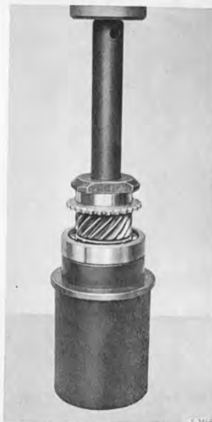
PRESSING ON THE BALL BEARING
