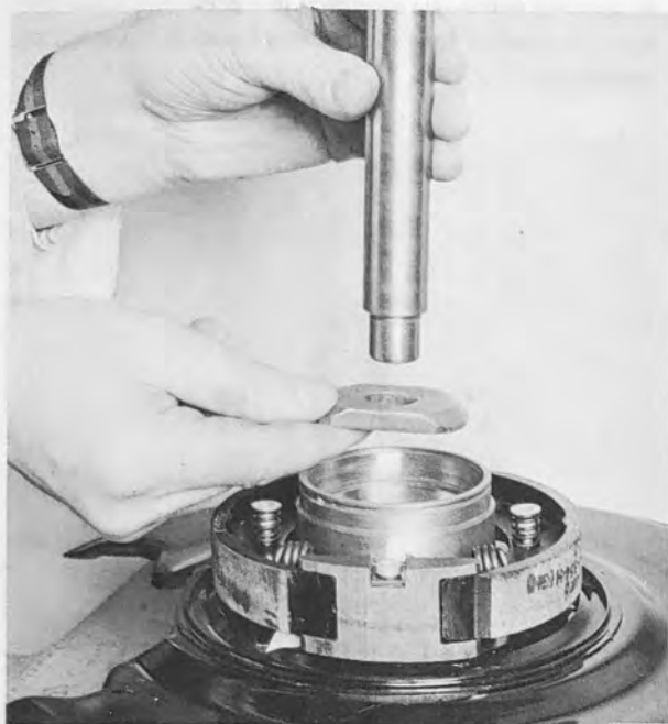
REMOVING THE OUTER RINGS OF THE BEARINGS Tool 839029
