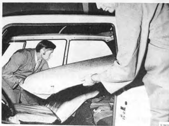
THE LINING IS MOVED IN POSITION
