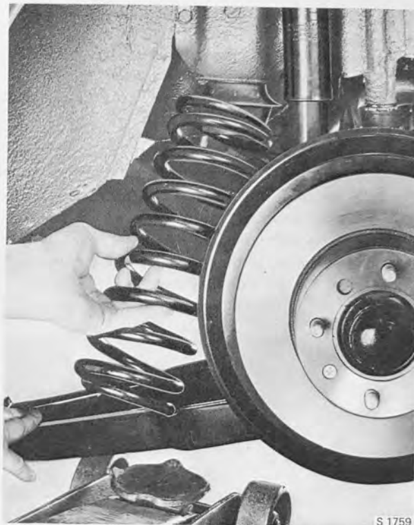
LOCATION OF COIL SPRING
