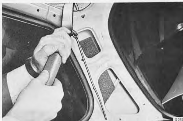
HOOKING THE HEADLINING TO THE REAR CORNERS Tool 829057
