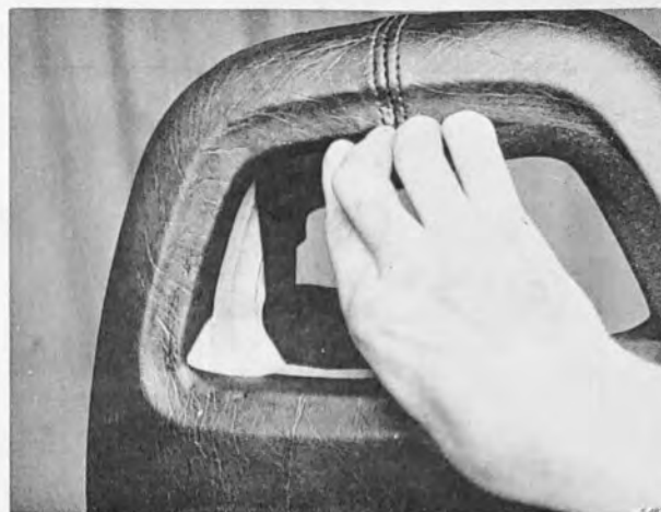
THREADING THE PLASTIC RING OUT FORWARDS
