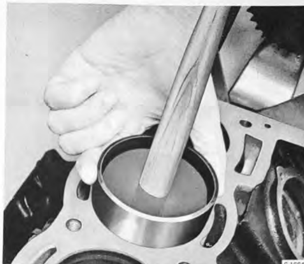
INSTALLING A PISTON
