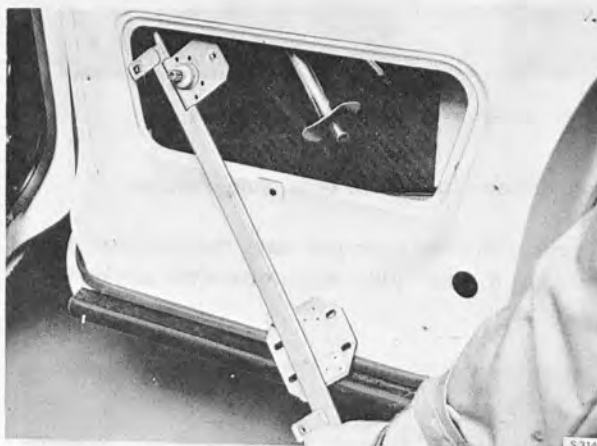
REMOVING THE REAR-DOOR WINDOW REGULATOR
