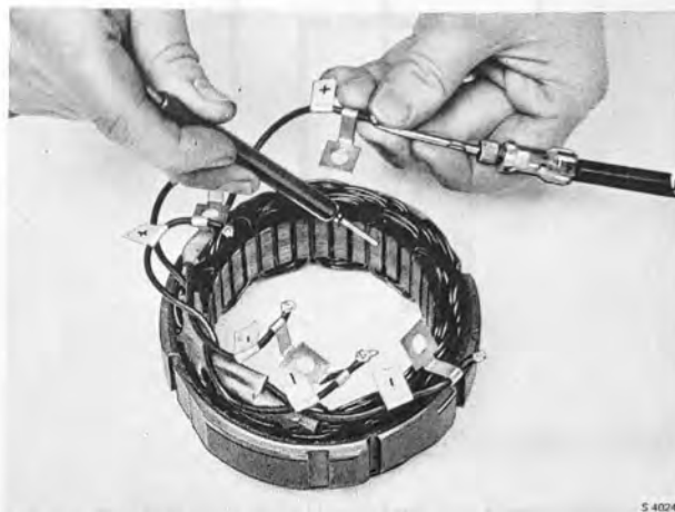
TEST OF STATOR WINDING
