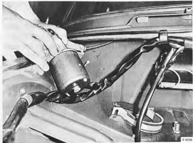
REMOVAL OF WIPER MOTOR AND FLEXIBLE CABLE
