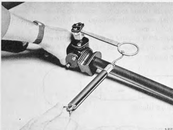
CHECKING THE STEERING GEAR TORQUE Tools 839013, 899528 and 899560
