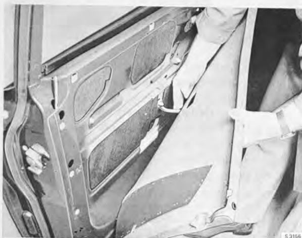
REMOVING THE DOOR TRIM
