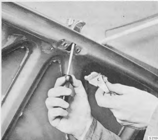
REMOVING THE LOCK FROM THE TRUNK LID
