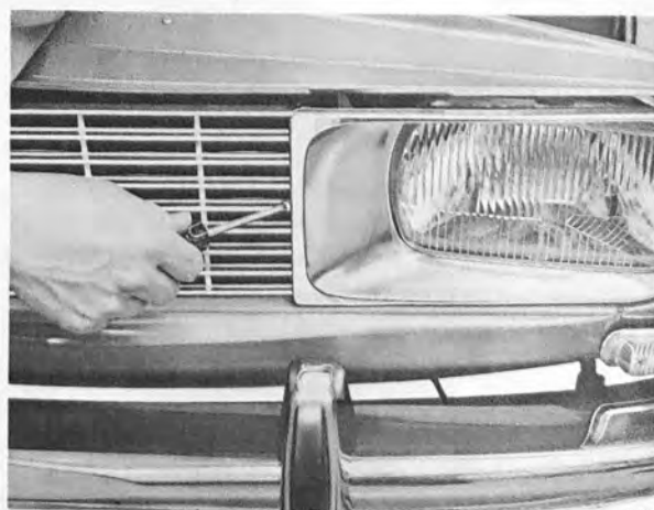
REMOVING THE TRIM FRAME
