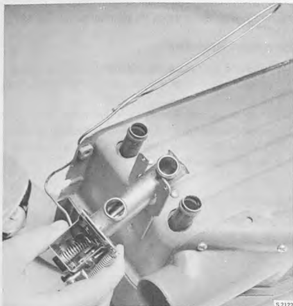
LIFTING OFF THE WATER VALVE
