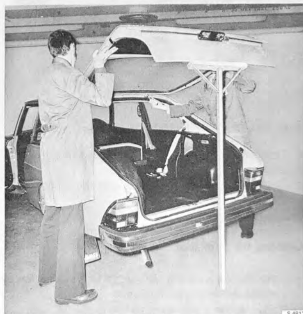
LIFTING AWAY THE TRUNK DOOR
