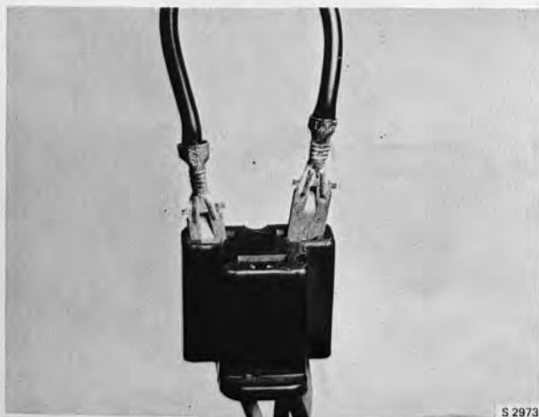
TERMINALS DF AND D+ CONNECTED
