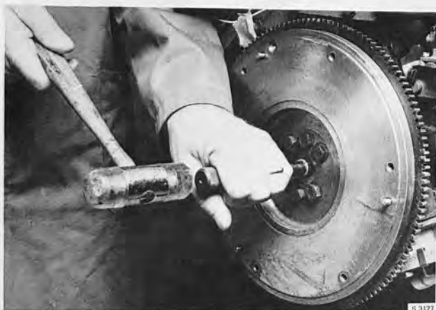
REPLACEMENT OF DISC-SHAFT BUSHING Tool 839206
