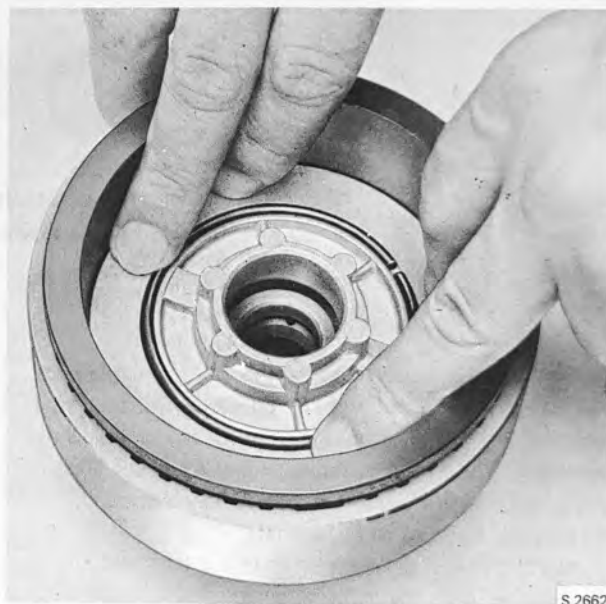
INSERTING PISTON IN FRONT CLUTCH Tool 879010
