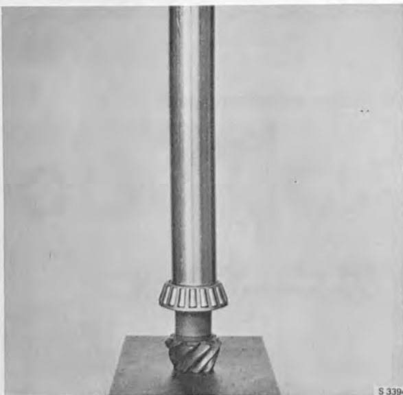
PRESSING ON THE ROLLER BEARING NEAREST THE PINION GEAR Tool 839014
