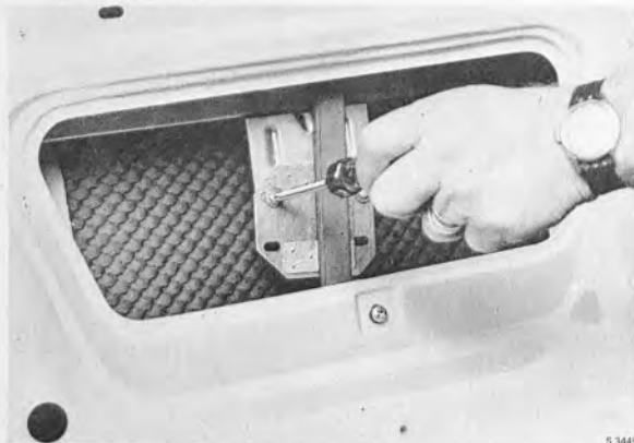
REMOVING THE SCREWS FROM THE WINDOW PANE RETAINER
