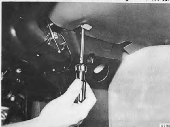
REMOVING THE RETAINING SCREWS FROM THE HEAT EXCHANGER CASING
