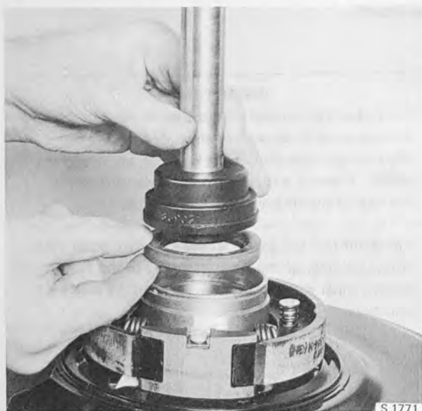
PRESSING IN THE SEAL RING Tool 839031
