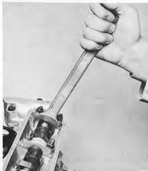
ROTATING THE CAMSHAFT WITH CYLINDER BLOCK REMOVED FROM ENGINE
