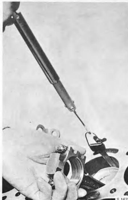
MEASURING PISTON CLEARANCE
