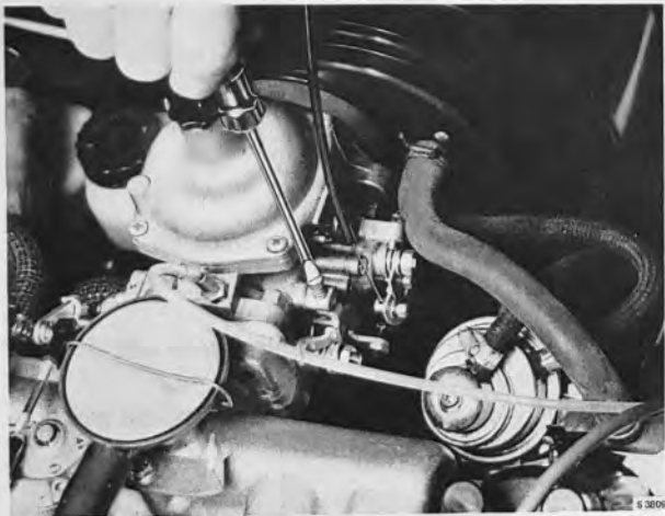
ADJUSTMENT OF IDLING SPEED
