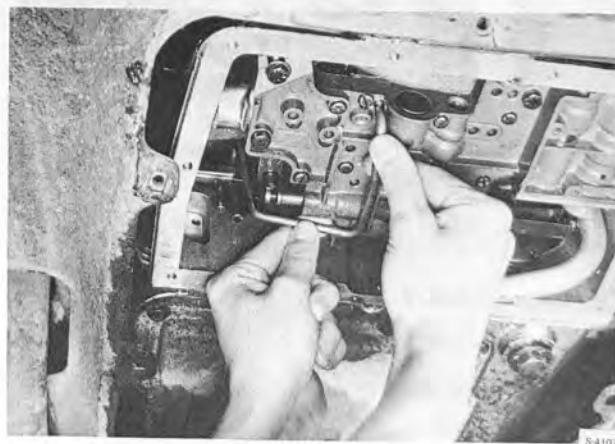
PIPE NO. 4 IS INSTALLED
