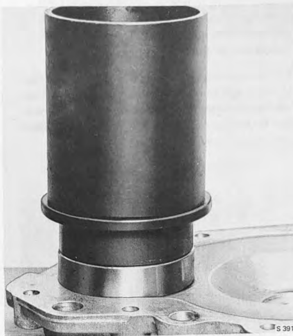
PRESSING ON THE GEAR AND BALL BEARING Tools 839009 and 839024
