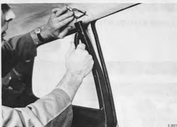
DOOR PILLAR PADS ARE MOVED INTO POSITION
