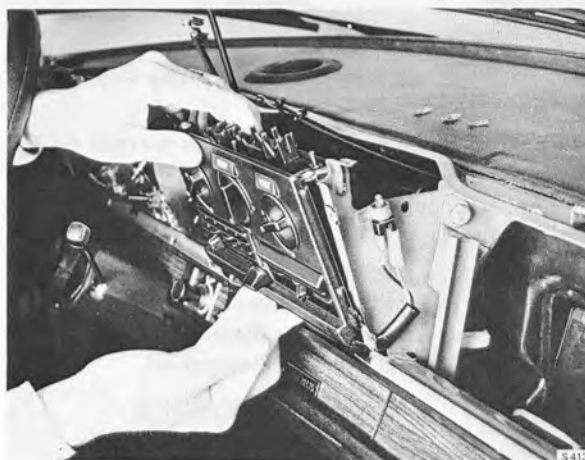
REMOVING THE HEATER CONTROLS, MODEL 1974
