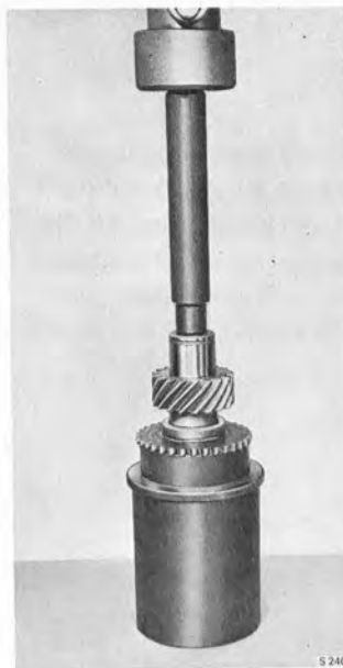
PRESSING ON THE FREE WHEEL DRIVER GEAR Tools 839009, 839018 and 839024
