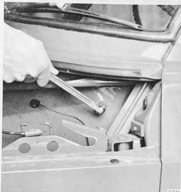
REMOVING THE INSTRUMENT PANEL RETAINING SCREWS
