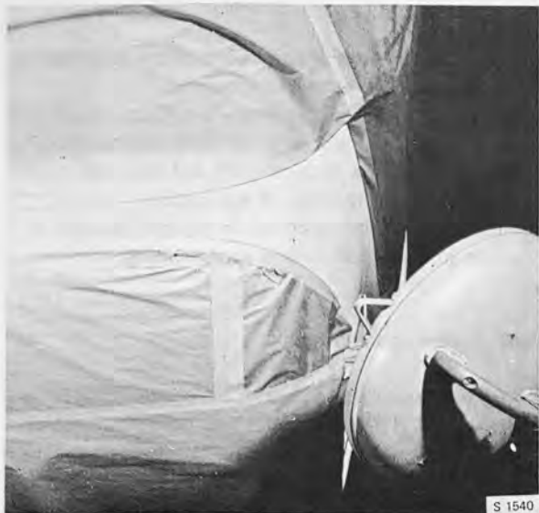
USE OF RADIATION LAMP TO DRY REFINISHED PART
