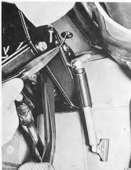
CONTROL WIRE LOOSENED FROM ACCELERATOR PEDAL
