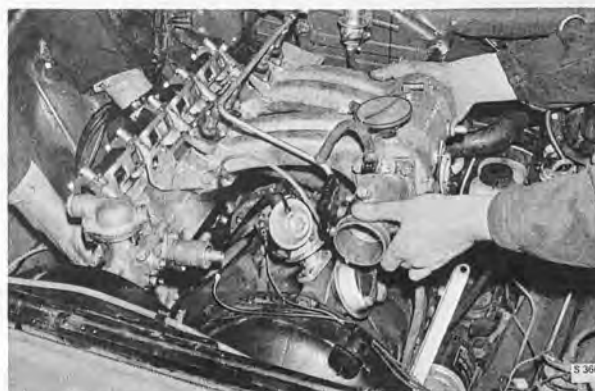
LIFTING OFF THE CYLINDER HEAD
